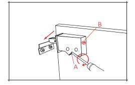
Screw A adjusts the height of the unit
